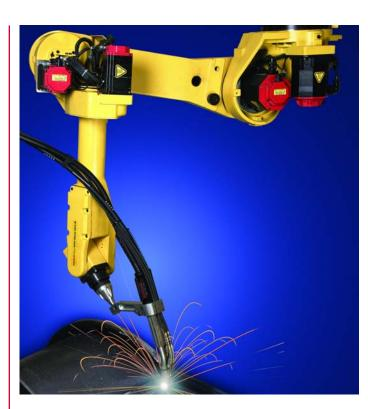
This data can be "played back" on consecutive passes, with the MP offset added to make preprogrammed adjustments in weld length, placement, and torch and work angles.
